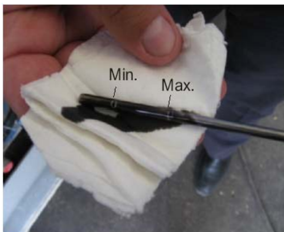
Cantitate de ulei in exces in baie
